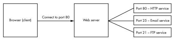
Figure 3-3: Ports allow servers to provide multiple services. Port numbers help forward client requests to the right service.
